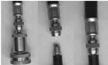
● Screw the small head onto the Schrader valve.
